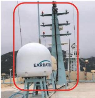
Too close to the mast, the antenna may be obstructed at mast direction.
