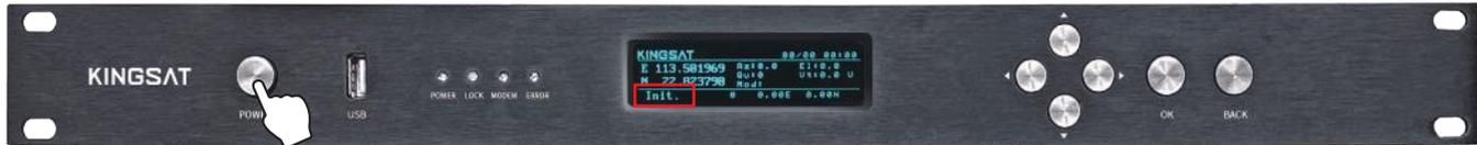
► *Error may happen as below shows. This means ACU can not communicate with antenna correctly. Please check all cable connections(whether the TX and RX coaxial cables are connected wrongly, or whether the F-N RF heads are tight) and restart system.*
