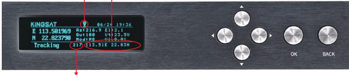
The azimuth angle calculated according to the GPS data of the fixed station.
