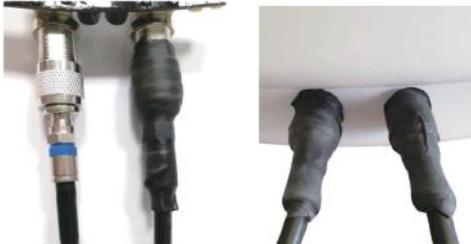
Connectors should be sealed with waterproof tape
