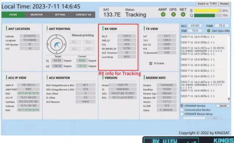
Check ACU side, press Right button, check RX VIEW page. Check whether all Rx parameters are correct or not.
