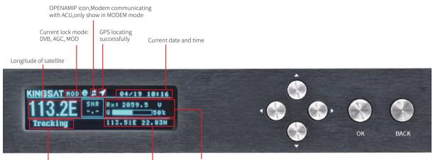
Current status of the antenna(ADU): 1.Init.: Antenna initializing 2.Search: Antenna searching satellite 3.Tracking: Antenna tracking satellite 4.Loss: Signal loss, quick troubleshooting see page 80 5.Error: Communication error, followed by an error code, For more information, see page 58 Rx parameters for Tracking Q, Quality of signal
