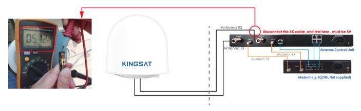
4. If the voltages of Tx and Rx coaxial cable are normal, but the status still shows Init or COMM ERROR, check the ACU mainboard or the antenna mainboard. Mainboard issues need to contact the manufacturer with help.
