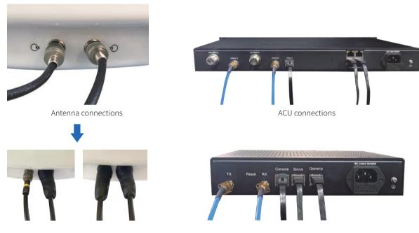
Connectors should be sealed with waterproof tape
