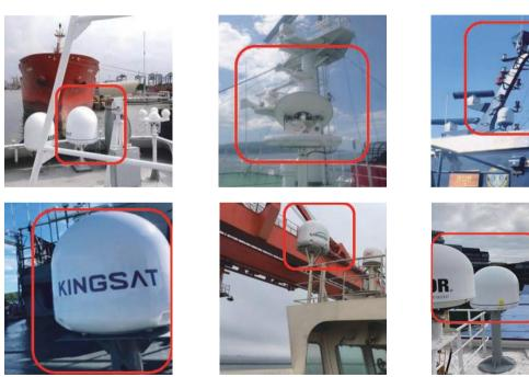
Too close to the mast, antenna can not get 360° free view to sky. The site needs to be re-selected, must be far away from obstructions while the height of mounting bracket should be made as high as possible.
