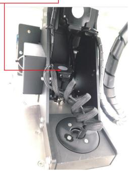
**E03** Skew motor issue. Check if SK motor is stuck, or belt of SK motor is broken or the connector of polarization switch is loose.
