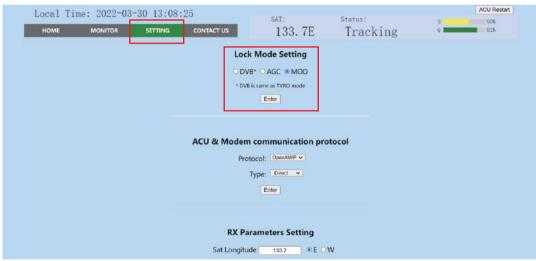
**Another way for setting Lock mode**, go to ACU, Press ok---Set Lock Mode, then BACK and SAVE.
