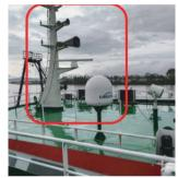
Too close to the mast, the antenna may be obstructed at mast direction.
