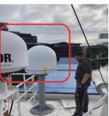
Too close to the mast, antenna can not get 360° free view to sky. The site needs to be re-selected, must be far away from obstructions while the height of mounting bracket should be made as high as possible.
