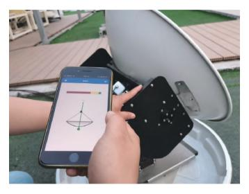
Step2. Moving the antenna by hand, better only move the azimuth direction because AZ and SK angel already fixed by initialization.
