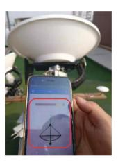
Step 4. Confirm whether the automatic alignment direction of the antenna and the pointing direction of the SAT finder application are consistent
