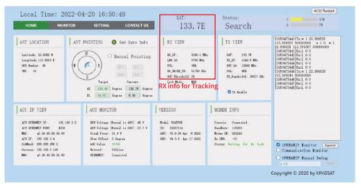
Check ACU side, press Right button, check RX VIEW page. Check whether all Rx parameters are correct or not.
